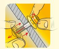
First put the screw through a flathead washer (if you are using one) and insert it through the protective guard you want to attach. Then put the Savetix® washer onto the screw from behind and screw the protective guard into position on the housing or frame.
