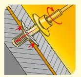
The Savetix® washer gets flattened during this process, making the hole smaller than the diameter of the threaded part of the thin-shank screw.
