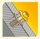
This deformation means that Savetix® has reduced the inner radius of the screw-hole so that the threaded part of the screw cannot fit back through the hole in the Savetix® washer or the protective guard.
